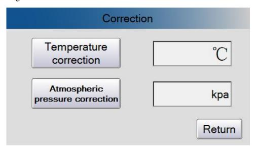
**Temperature correction:** using the glass thermometer which has been calibrated, to test the temperature of the same sample, and then compare the actual temperature value and measurement temperature value to obtain the difference. Then input it to modify the corresponding temperature correction value.
