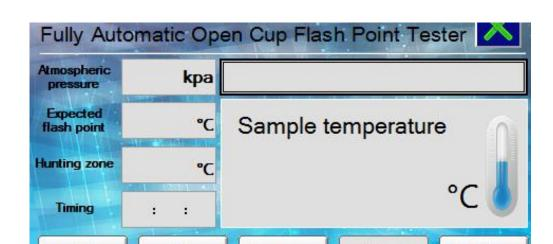
Before starting to run the test, be sure to set the parameter values: expected flash point and hunting zone. Through special gas pipe to connect with gas device used in experiment, please pay attention to the seal of connection pipe, which is forbidden to leak.
