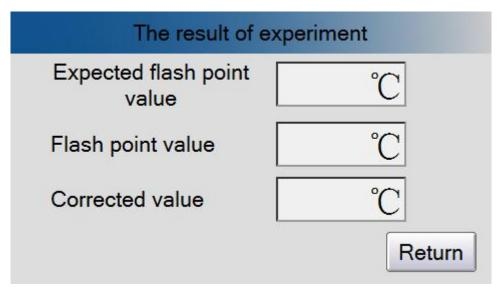
When you detected the flash point value, the result of the measurement will showed on the screen automatically: When the result of the flash point and the flash point which was corrected by the barometric pressure showed, the buzzer rings at the same time.
